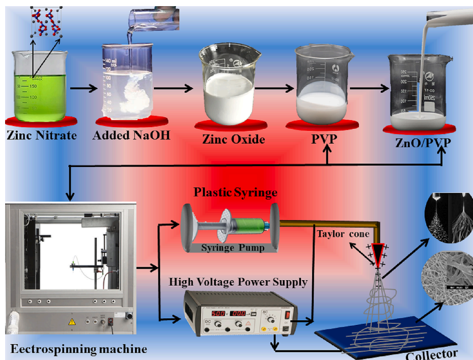
Fig. 1. Synthesis of PVP/ ZnO obtained for electro spinning method.
