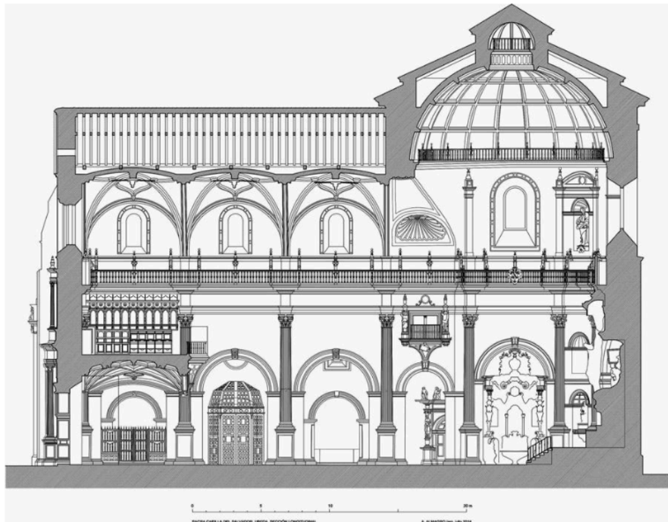
Figure 12. Longitudinal Section of the Sacristy of the Sacred Chapel (Note: By the author Almagro, A., 2014, drawing of the Saviour in Úbeda.)
