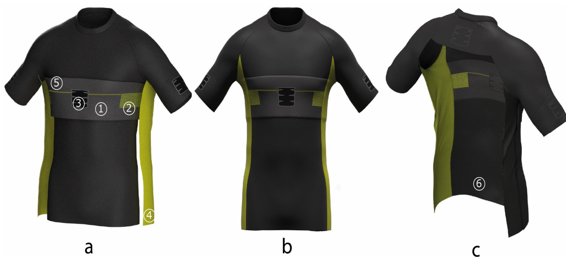
Figure 2. (a) Textile patterns from Figure 1 being assembled to fabricate the T-shirt (inside-out view). (b) T-shirt already fabricated (inside-out view). (c) Cross-sectional view of the T-shirt. The building elements of the T-shirt are the following: 1. intarsia-knitted chest patch, 2. chest rectangular electrode pad, 3. ECG device pocket, 4. side textile electrode, 5. interconnecting conductive track, 6. interior side of the T-shirt fabric.
