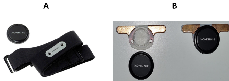
Figure 4. (A) Movesense Active with its chest strap delivered for ECG measurement. (B) Customized interface adaptor for Movesense Active device.
