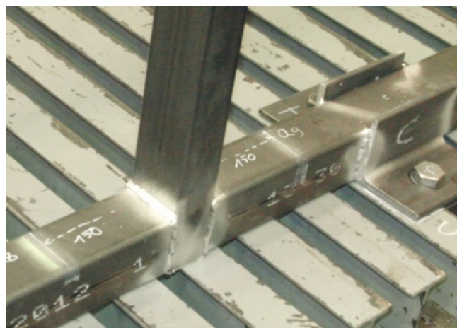
Figure 5. Clamping weld details.
