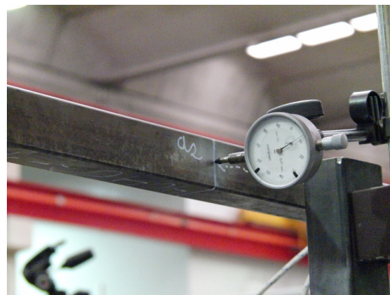
Figure 8. Mounting of the dial gauge for the displacement measurement of the a2 section.
