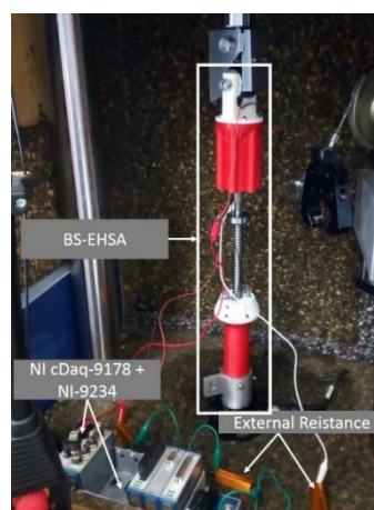
Figure 5. Bench test setup for the BS-EHSA.
